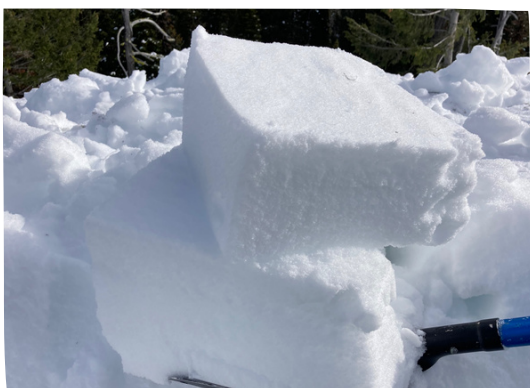
L-R: (1) In mid-Feb. wind stiffened snow popped off easily with a burp test, but did not propagate in ECTs (2) Faceting snow buried in the snowpack in early April (3) Volunteer Burket Kniveton inspecting the crown of a slab that failed on a persistent weak layer formed around a mid-Jan. crust
