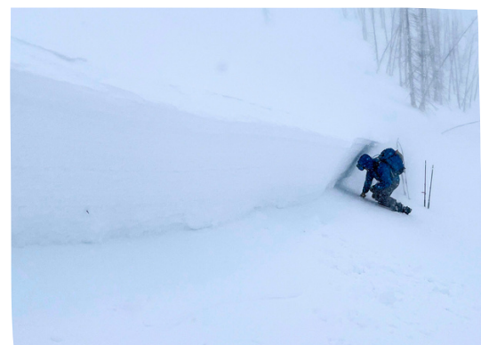
L-R: (1) In mid-Feb. wind stiffened snow popped off easily with a burp test, but did not propagate in ECTs (2) Faceting snow buried in the snowpack in early April (3) Volunteer Burket Kniveton inspecting the crown of a slab that failed on a persistent weak layer formed around a mid-Jan. crust
